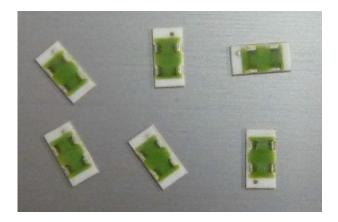
Typical Ceramic Strain Gauge
